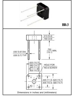
Single phase, half wave, 60 Hz, resistive or inductive load.
